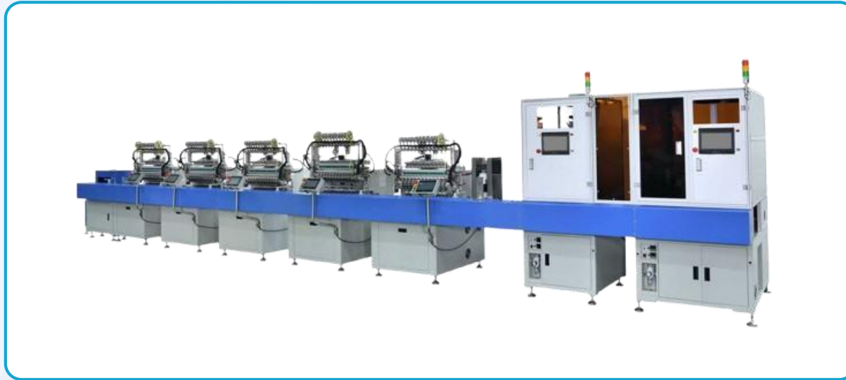
Automatic Laser Soldering Production Line for Winding and Basing of Transformer
